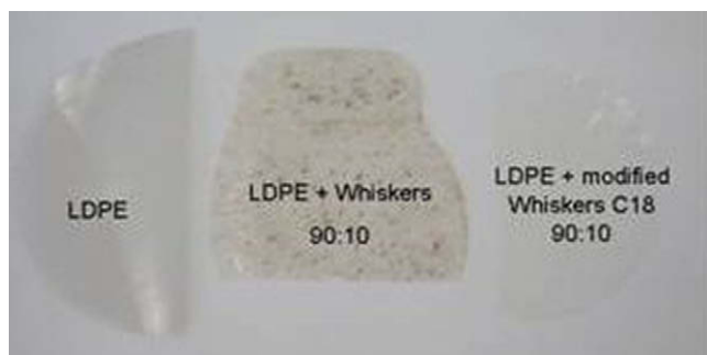
Fig. 10. Photographs of the neat film and ramie cellulose whiskers based nanocomposite films reinforced with 10 wt% of WRU and WRC18.
